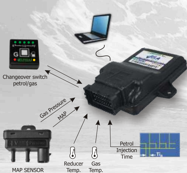
The VELA Freestyle Connection Schematics
